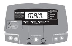
You control resistance and incline settings when you use the Manual Program. The profile begins as a flat line. Use the arrow keys to change the resistance or to adjust the ramp incline. The program profile reflects changes in all subsequent columns. The blinking column indicates your position in the program.
