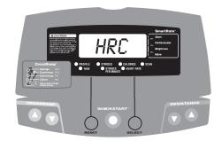
The Heart Rate Control Program lets you set a target for your heart rate. The program adjusts the resistance to maintain your heart rate within two beats per minute of the target heart rate while you exercise. To use this program, you must wear the chest strap so the program can monitor your heart rate throughout the session
