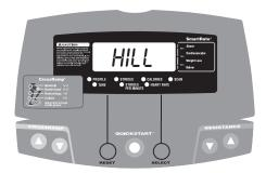
The resistance in the EFX5.19 Hill Climb Program is preprogrammed. To override the resistance settings for each column, press the RESISTANCE arrow keys. The changes raise or lower the columns on the remaining portion of the program profile.
